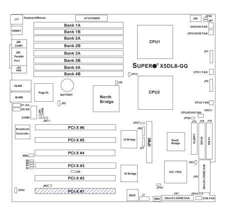
Note: DIP Switch 4 sets the CPU Core/Bus Ratio (see Section 2-7). CR5 is a power LED indicator (see Section 2-6). Jumpers not noted are for test purposes only. IPMI is optional.
